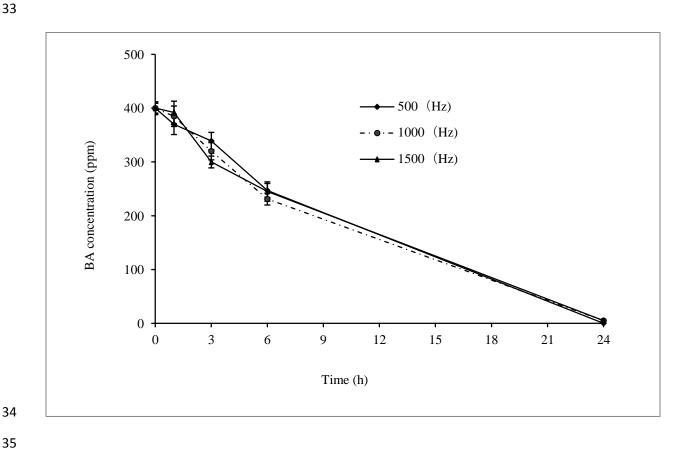
**Fig. 1.** Changes in benzoic acid concentration of the nutrient solution due to application of electrodegradation using alternate current (AC) at three different frequencies for 24 hours. Electro-degradation was applied in 10 L of 25% standard "Enshi" nutrient solution with 400  $\mu$ M L<sup>-1</sup> benzoic acid. The vertical bars represent SE (n = 5). In AC supply 50% duty ratio, about 2.0 ampere and 14.0 volt were maintained for all frequencies. (Experiment I)
